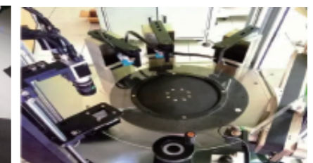
Visual guidance of screwing
