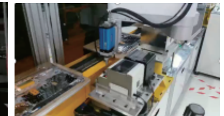
Visual guidance of loading for PCBA test loop
