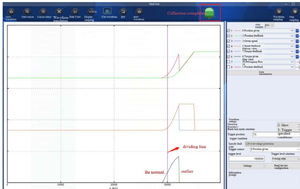
Figure 6.11.3-5 Analysis of Black Box Sampling Waveform
