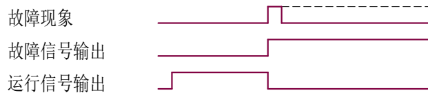
Figure 7-17 Fault signal timing
