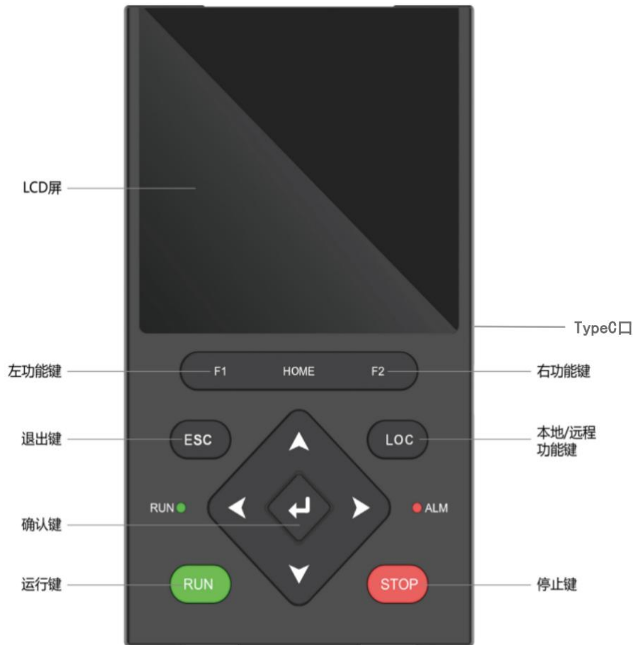
Figure 5-1 Names and functions of various parts of the operator
