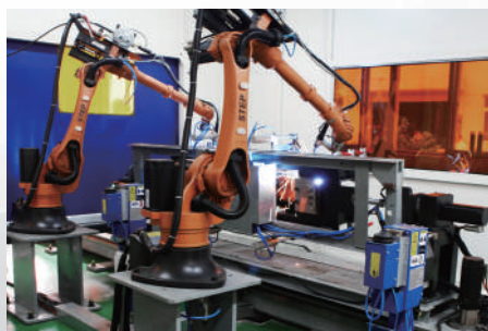
Enforce Beam (Elevator) Welding
