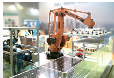
Solar Panel Handling
