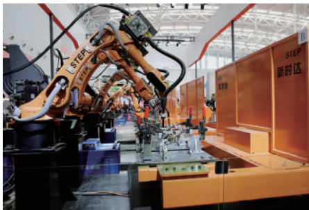
Car Frame Welding
