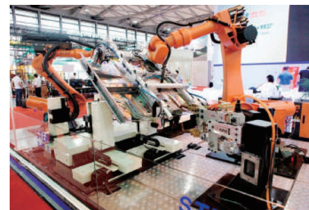
Car Frame Flexible Spot Welding
