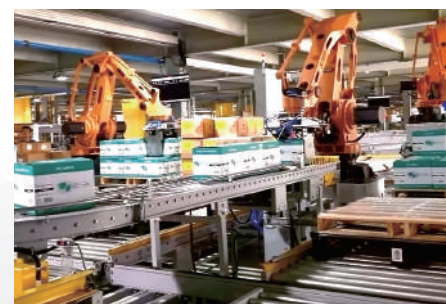
Pharmacy Production Line (Palletizing )
