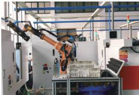
One Robot for Multiple CNC Machines
